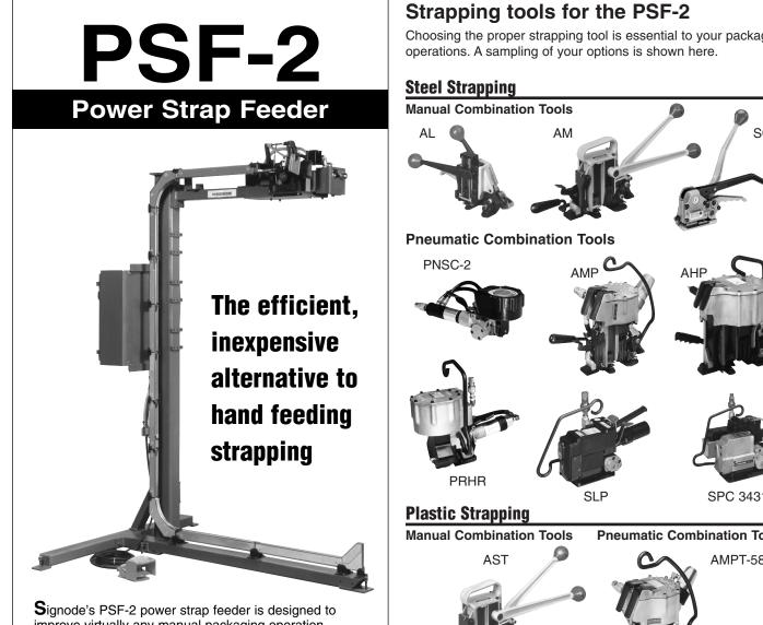
improve virtually any manual packaging operation regardless of package size, strapping material, pallet type, or packaging line configuration. Its modular design enables you to customize the PSF-2 to accommodate the unique requirements of your packaging operation. The PSF-2 features automatic strap feed shutoff and an automatic seal feed bend over device. Some popular options include: chute extensions, casters, pallet void feeding attachments, strap grippers and directors, and more.
